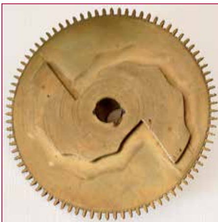
Figure 5 (below). The double-six snail on the reverse of the hour wheel of the Swansea Tompion
