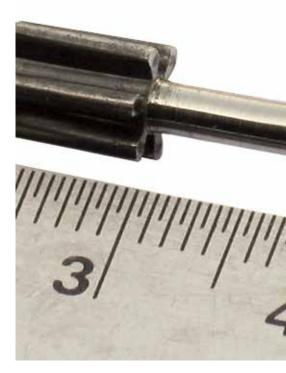
until the softened arbor end is located within the large hole of the brass re-pivoting tool.
